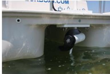
The Esc'KEY is propelled by a Minn Kota 112lb thrust motor that propels this 36vdc model at 4.5mph. It is steered by a comfortable and easily reached tiller handle mounted between the 2 helm seat cushions allowing either left or right side control of the boat. Forward and reverse speeds are dialed in with the simple easy to reach dash mounted knob. The motor is raised or employed in the stern of the boat by lifting or lowering the D handle on the motor tube.
